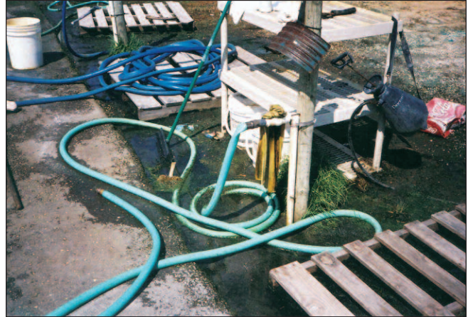
Figure 33: above: unsafe work area, runoff, erosion. below: Safe and clean, curbed, water captured by drain for proper disposal.
