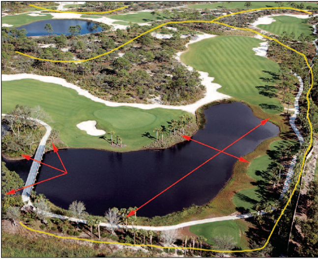
Figure 1: A typical golf course designed with the environment in mind. The yellow line shows wildlife corridors; the red lines point to water quality buffer areas.
